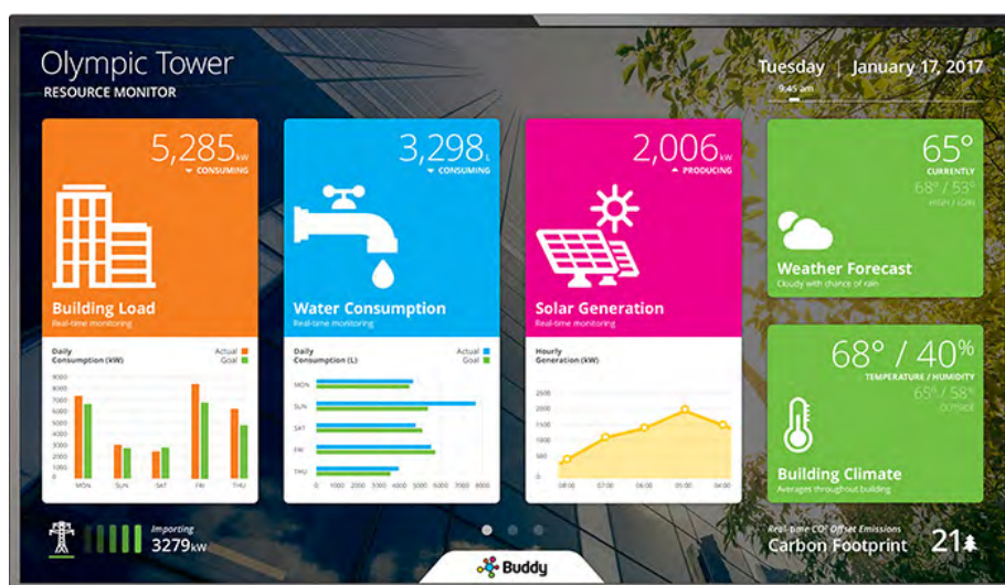
Occupant Facing Dashboard of BuddyOhm System
